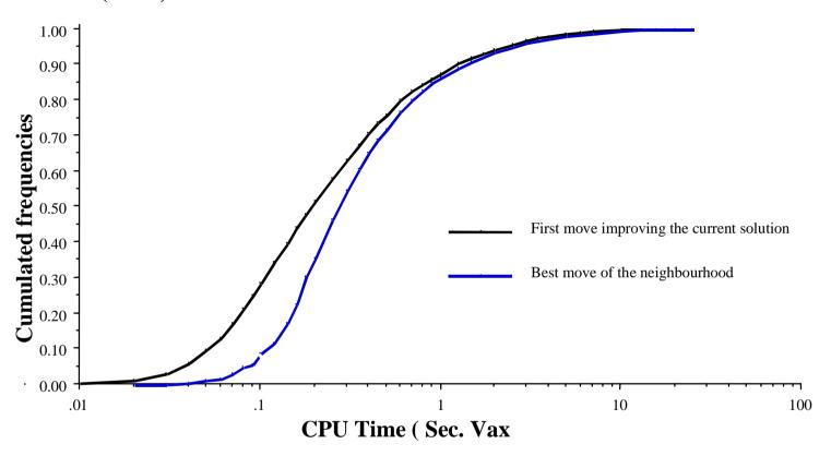
CPU time to find optimal makespan (permutation flow-shop, 9 Jobs, 10 Machines)
